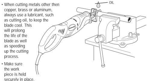
Hold smaller pieces, such as pipe or conduit, in a vise or attach to the workbench with clamps.
